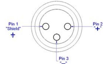
Fig. 1. XLR Output Connector Assignment of QTC50
